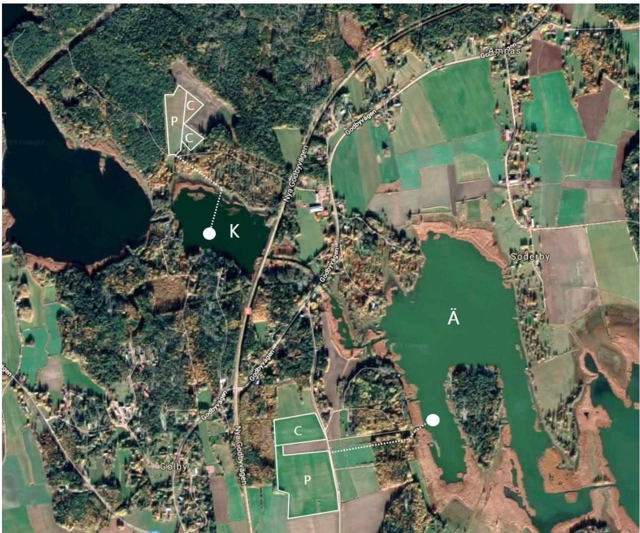
Figure 7. Kaldersfjärden (K) and Ämnäsviken (Ä) with the locations for irrigation water uptake (white dots). The fields near Kaldersfjärden and Ämnäsviken are marked with white lines. P = pilot area, C = control area. The dotted white lines represent the water pipelines.
